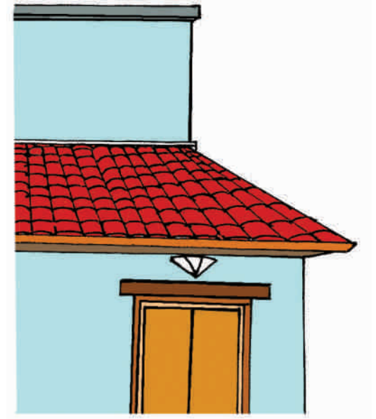
Earthenware Or Designer Tiles Can Be Used For Insulation Of Sloping Concrete Roofs
