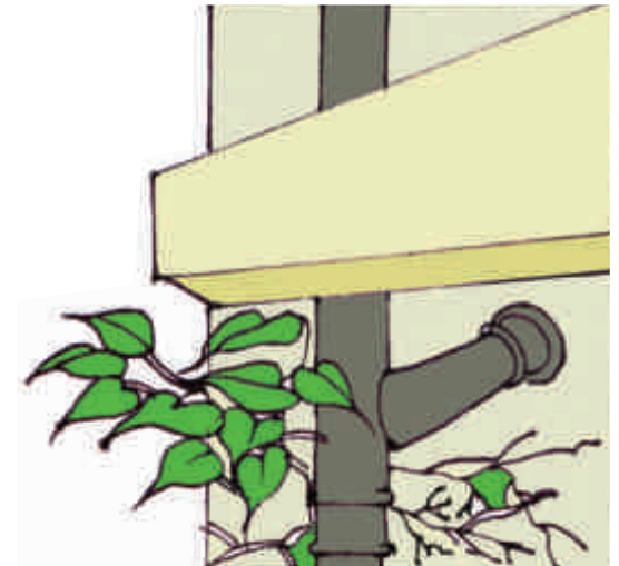
Plant Growth Can Lead to Cracks
