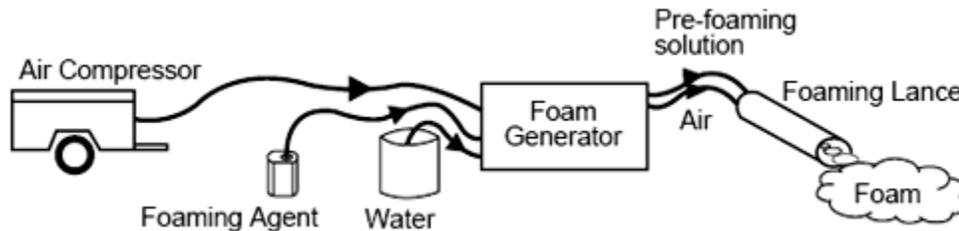
Making foam from foaming agent, water and compressed air.
