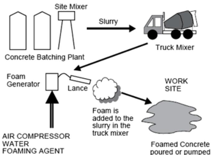
A Schematic diagram showing the stages involved when making foamed concrete.
